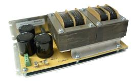
The PSA80V4A-1 power supply has a single 80V output, a voltage input of 115 or 220VAC, and power capabilities of up to 320 watts. With an unregulated output and a size of 8.30" x 4.25" x 2.81" and dual mounting position "L Bracket," the PSA80V4A-1 can be mounted just about anywhere. The PKG-232-MBC08-PS-CBL includes two wires for powering the MBC082561.
